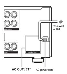
\* The configuration, shape and number of AC outlets vary according to the area code.
